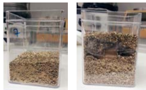
Fig.02: Placement of test product (wood in LDPE film) in test container (left) with consequent burial in substrate (right).
